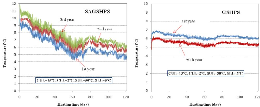
Figure 9 Fluid temperatures out of evaporators of HP of SAGSHPS and GSHPs
