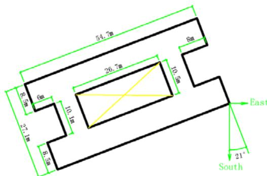
**Figure 1 Shape and orientation of the ECLC building (dimensions in meter)**
