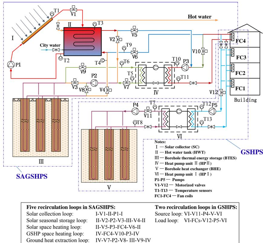
Figure 2 Schematic of the HSGSHPS
