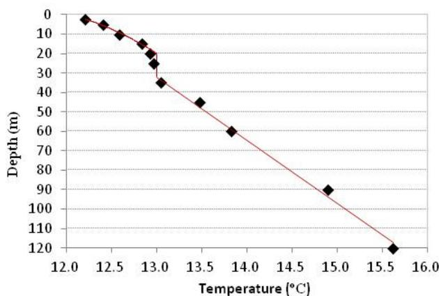
**Figure 3 Undisturbed temperature of soil with depth of boreholes in winter**
